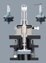
Low operating and maintenance costs are assured by the well proven Axial Flow Valve. Reliable, simple and effective and based on a flexible expanding sleeve, the Axial Flow Valve has no moving parts to stick, wear or break.
